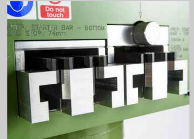
Whilst the multi-head tool is more complex and expensive than single-function tools, the need for time-consuming tool changes and multiple punch stations, is dramatically reduced.
