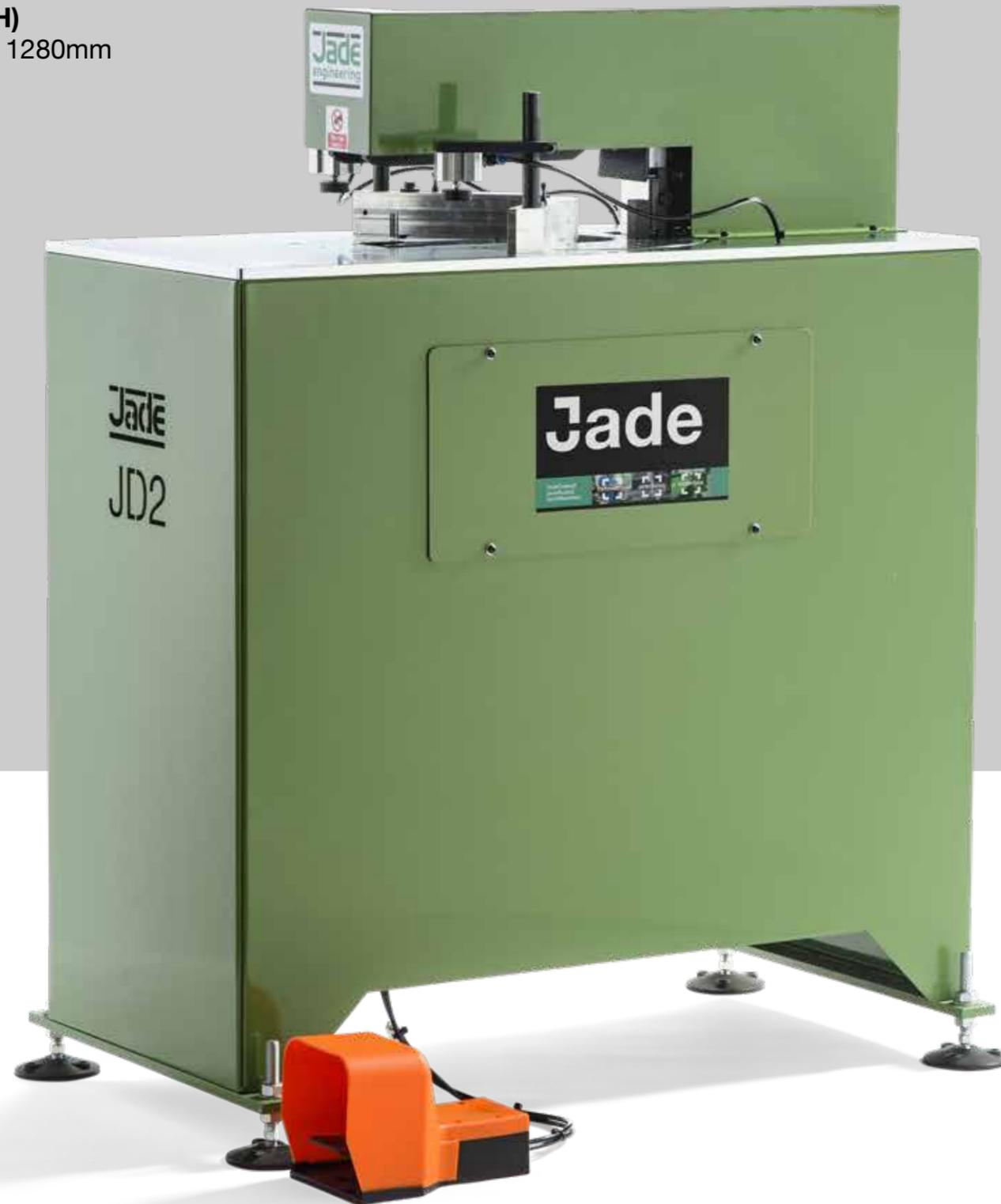
The JD2 Groover allows the fabricator to clean the excess weld sprue on the top and bottom faces of either reverse butt or corner welds. The JD2 comes equipped with adjustable back fences which can be easily rotated from 180° to 60°. There is also a fence setting which allows the user to clean cruciform welded joints. The JD2 is a floor standing machine operated by foot pedal and comes complete with top and bottom knives to customer's specification.
